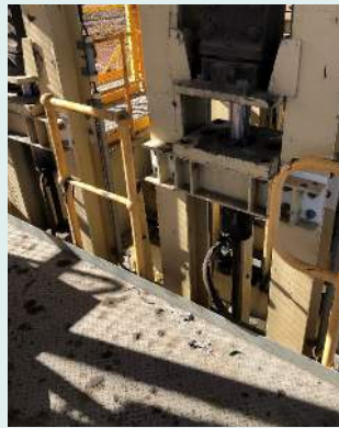
Walkway providing access to a machine—AS 4024.2201-2204 applies
